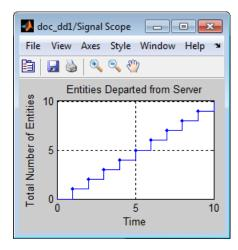
After an entity departs from the Single Server block, the block updates its output signal at the **#d** port. The updated values are reflected in the plot and highlighted with plotting markers. From the plot, you can make these observations:
