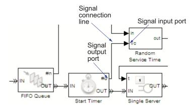
In a discrete-event system, the signal input port coming into a block changes to an empty arrow when you perform update diagram:
