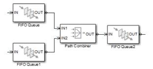
• **Connecting a feedback path:** A feedback path enters the same queue as an ordinary path.
