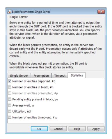
Then click **OK**. The Single Server block acquires a signal output port labeled #d. During the simulation, the block will produce an output signal at this #d port; the signal's value is the running count of entities that have completed their service and departed from the server.
