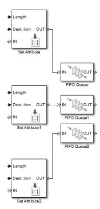
The queue uses a FIFO queuing discipline, which does not take into account the destination of each packet. Note that such a model can suffer from "head-of-queue blocking," which occurs when a packet *not* at the head of the queue is forced to wait even when its destination is available, just because the packet at the head of the queue is aiming for an unavailable destination.
