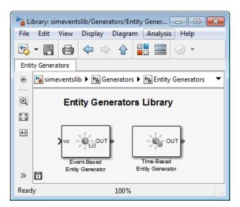
**2** Drag the Time-Based Entity Generator block from the library into the model window.
