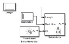
The packet generation processes for the different sources differ only in the initial seeds for the random number generators and the values for the source attribute.
