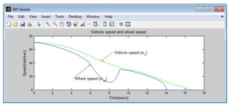
By comparing these plots with the plots in "Lesson 1: Run the Time-Based Model" on page 2-30, you can see that the delay introduced between the ABS controller and the braking system significantly degrades the performance of the braking system:
