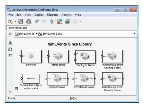
**8** Drag the Signal Scope block and the Entity Sink block from the library into the model window.
